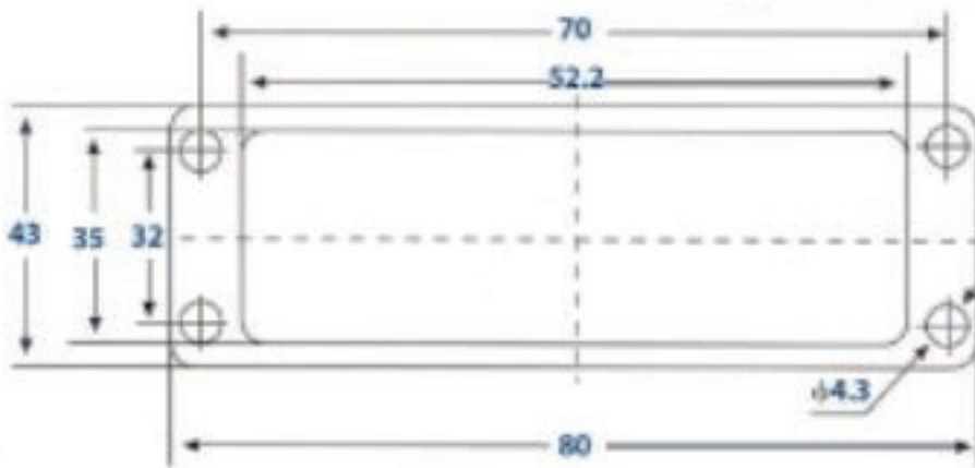
Mounting Dimensions (mm)
