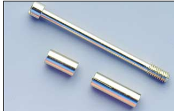
FVS/VCE cat. No. FV108 Screw and sleeve to perform the internal link between the front and back conducting bodies of FVS.4 terminal blocks
