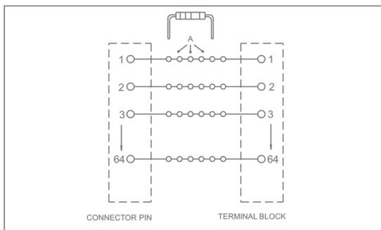
Component mounting holes located on each trace at 0.1" centers allow customers to insert components in parallel or series. To place a component in series customer removes trace (A) between component mounting holes under added component. The traces are located on the bottom side of the printed circuit board.
