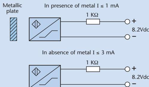
The NAMUR sensors are electronic devices whose absorbed current varies in the presence of a metallic object. The difference between these sensors and traditional sensors is the absence of amplifier trigger stages.
